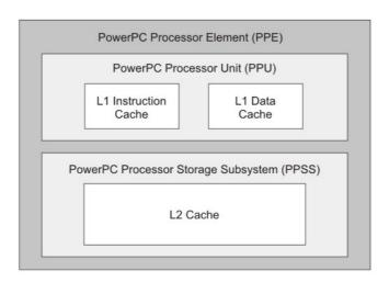
The PowerPC Processor Element (PPE) is a general-purpose, dual-threaded, 64-bit RISC processor that conforms to the PowerPC Architecture, with the Vector/SIMD Multimedia Extension.
