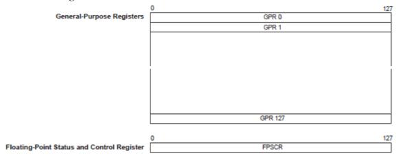
This section describes the Synergistic Processor Element (SPE) user registers. The complete set of SPE user registers is shown in Figure. All computational instructions operate only on registers—there are no computational instructions that modify storage.
