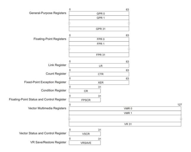
Floating-Point Registers (FPRs) – The 32 FPRs are 64 bits wide. The internal format of floating-point data is the IEEE 754 double-precision format. Single-precision results are maintained internally in the double-precision format.
